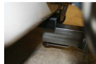
Carrier Latch Pin Engaging to the Carrier Latch Pin Receiver
